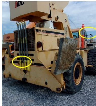
Cameras are mounted at blind spots with a monitor in the cab for the driver to see.
